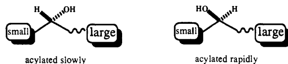
Figure 1. Simple model for predicting which substrates will be resolved effectively via biocatalytic acylations mediated by crude lipase from Pseudomonas sp. (Amano AK) and the sense of the enantioselection.
